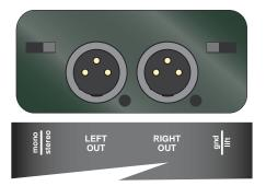
Stereo/Mono When in stereo the units left and right are separet. When in Mono The left and right inputs are combined together. In mono mode you can plug a single left or right input into the DB24 and you will get output from both left and right.
